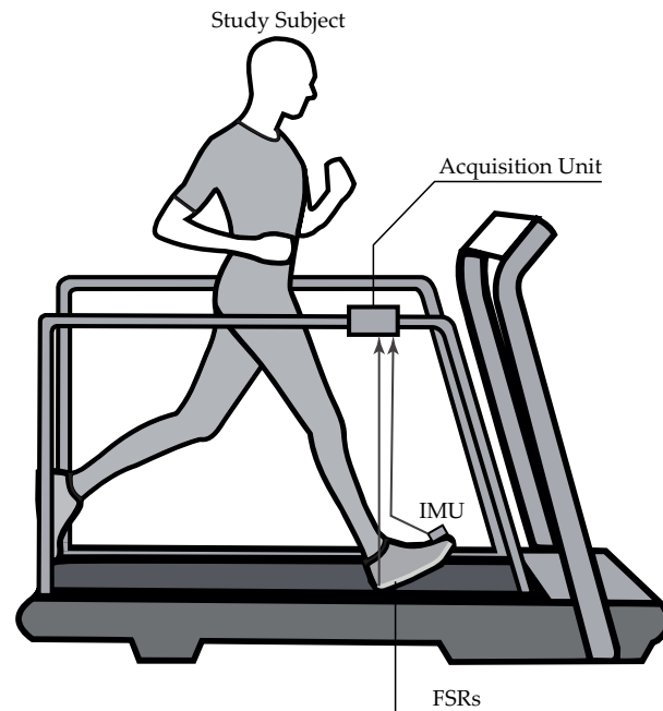
Figure 6. Experimental setup. Each subject was instrumented on their dominant/affected side with a custom FSR-equipped insole and an IMU placed on the dorsal side of their foot. Foot motion data were captured by using a Raspberry Pi running ROS to ensure synchronized data acquisition.
