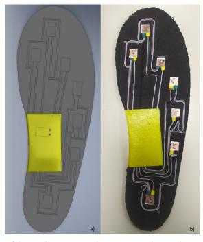
**Figure 5.** (a) 3D design of the insole in AutoDesk Inventor Professional 2018. (b) Inside view of the insole with custom-made capacitive sensors located at the main support plantar points.
