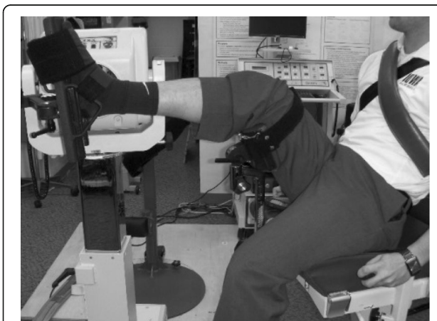
Fig. 1 Experimental set-up for ankle strength testing using the Biodex isokinetic dynamometer with the knee flexed and ankle elevated
