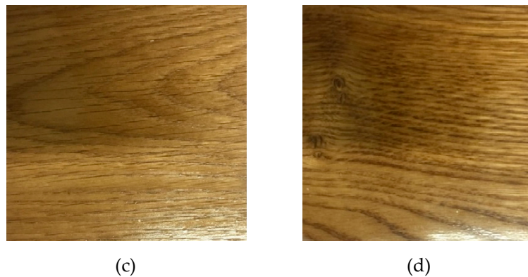
Figure 1. Images of PUA coating and its coated oak samples at different coating amounts. (a) PUA coating; (b) 12 g/m 2 PUA coated oak; (c) 60 g/m 2 PUA coated oak; (d) 120 g/m 2 PUA coated oak.
