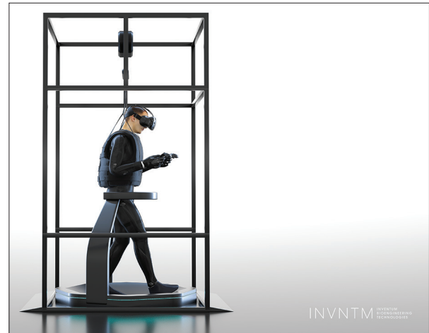
Figure 3: The user will be using either the Vive® or Rift® head-mounted display while strapped into the body harness of the IH-GAIT Frame Model. This setup allows both upper and lower-body interaction with the VR environment using either the Vive® vibration feedback controllers or Oculus Touch®, and the Virtuix Omni™ locomotion simulator
