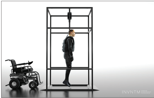
Figure 2: User will be strapped into the body harness of the IH-GAIT Frame Model to maintain a standing position. The user will wear either the Vive® or Rift® head-mounted displays. This setup allows upper-body interaction with the VR environment using either the Vive® vibration feedback controllers or Touch®
