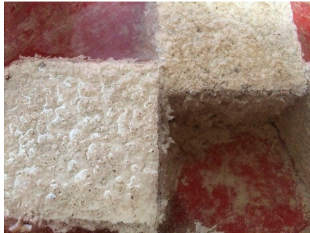
Figure 6. Physical appearance of typical samples in 5% sulphuric acid solution.
