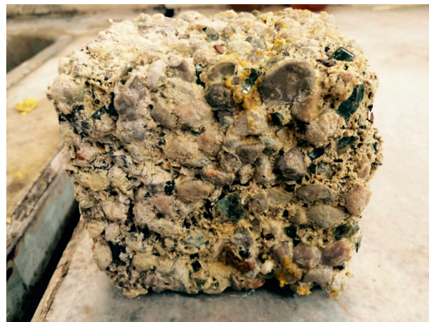
Figure 7. Physical appearance of typical samples after immersion in 5% sulphuric acid solution.
