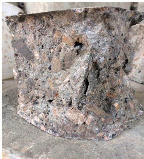
Figure 2. The fractured face of a sample containing 10% zeolite and 15% tuff after compressive strength test.
