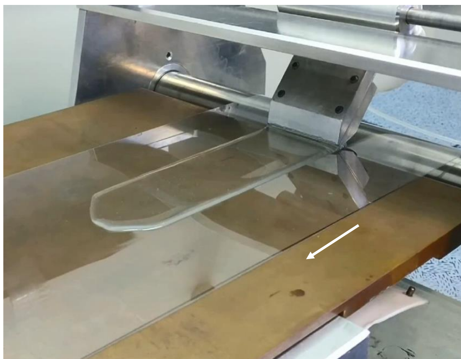
Figure 2. A photograph of slot-die roll to roll machine shown depositing a Chi-TEOS IPN hydrogel onto a PET substrate over a hotplate. The arrow shows the direction of travel.
