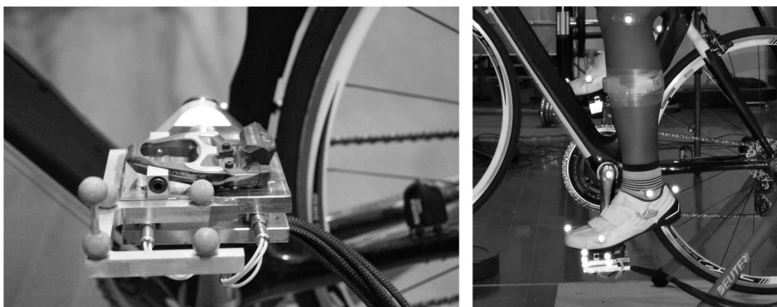
Figure 1. Image of the instrumented pedal force system with cleat fixed on the pedal.
