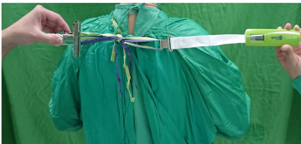
Figure 3. Fastening the ties with a tightening force reaching 1 kg.
