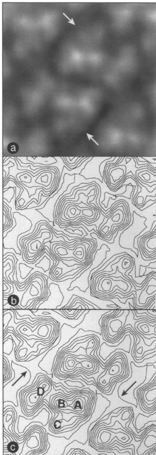
Figure 4. (a) Density map of the average obtained from the 268 nm defocus images. Symmetry has not been imposed, nor has this average been filtered. The high degree of twofold symmetry is clearly evident. Slight asymmetry was consistently noticed in the areas indicated with arrows. (b) Contour map with no symmetry imposed, filtered to 1.7 nm, for comparison with the symmetrized contour map (c). (c) Contour map of the average after filtering to 1.7 nm. Twofold symmetry has been imposed. The unit cell was 11.4 \times 17.0 nm. Individual areas of density within the monomeric unit are indicated by A–D. Arrows indicate crystallographic connections between the unit cells.
