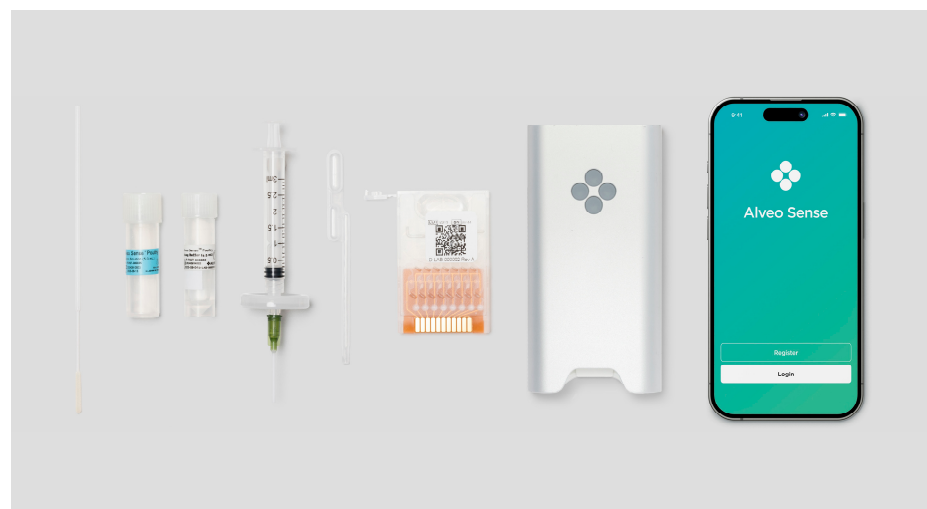
Figure 1. Components of the Alveo Sense Poultry Avian Influenza Test. The test components include the following (left to right): PurFlock Ultra swab, Alveo Sense Poultry Avian Influenza Swab Elution Solution vial, Alveo Sense Poultry Avian Influenza Assay buffer vial, Alveo Sense Poultry Avian Influenza Syringe Filter, transfer pipette, Alveo Sense Poultry Avian Influenza Type A H5, H7, or H9 cartridge, Alveo Analyzer, and Alveo Sense Mobile Application.
