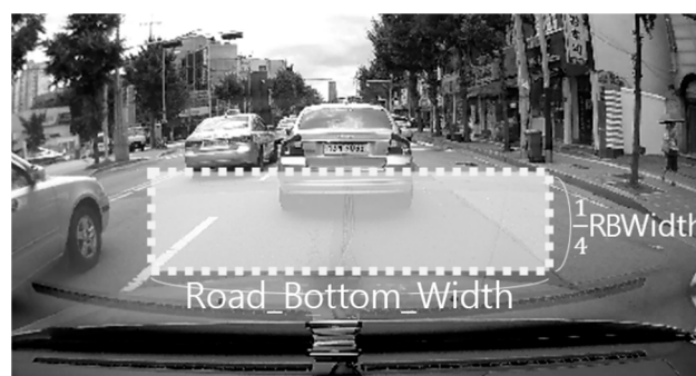
Figure 6. Predefined ROI when failing to detect the car shadow.
