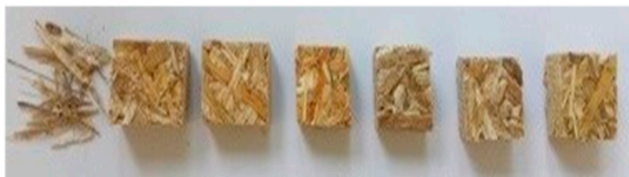
Figure 1. The samples (from left to right): rape straw, epoxy sample, epoxy-H 2 O sample, epoxy-NaOH sample, glue-LS sample, glue-LS-H 2 O sample, glue-LS-NaOH sample.
