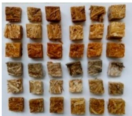
Figure 2. The photo of the samples covered by molds after finishing of the test (from top to bottom): glue sample, glue-H 2 O sample, glue-NaOH sample, epoxy sample, epoxy-H 2 O sample, epoxy-NaOH sample. The first three samples (from top to bottom) were sterile and the other three samples were nonsterile in each line. All samples contained straw.
