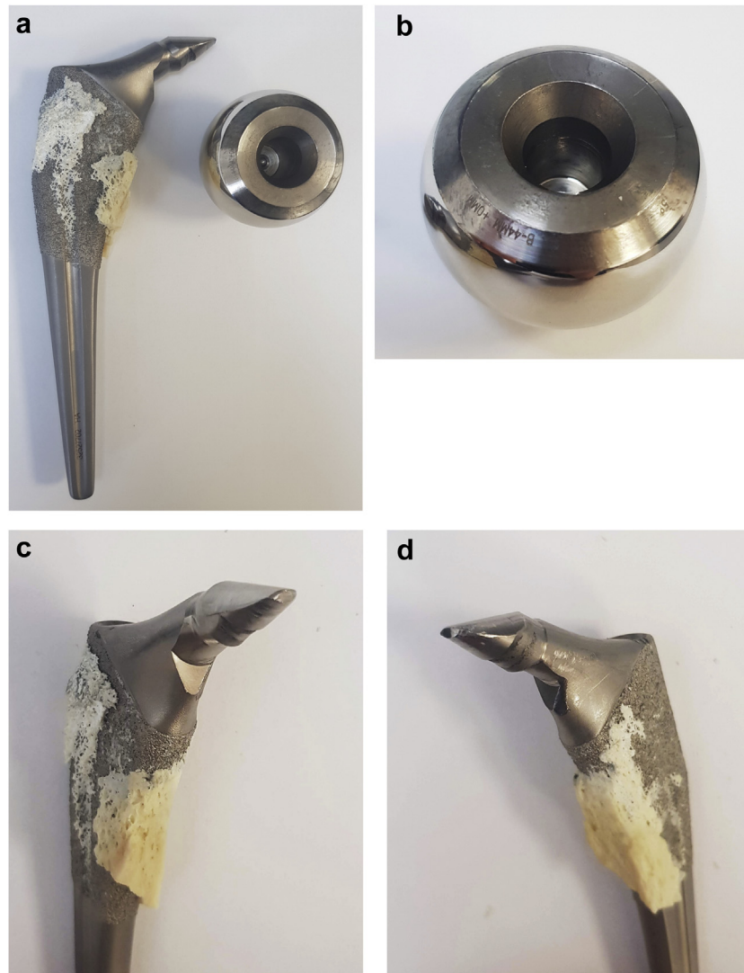
Figure 2. (a) The recovered accolade TMZF explant showed severe corrosion of the modular junction and corrosion of the medial portion of the femoral neck. (b) There was no increased wear visible inside or outside the size 44/0 cobalt-chrome head. (c, d) Rotational views of the recovered explant demonstrate the extent of corrosion present without fracturing of the stem.
