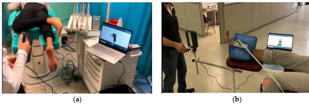
Figure 2. Scanning of the foot without any foot locking system and a handheld 3D scanner (a), and scanning of the foot with a foot locking system and a tripod for the 3D scanner (b).
