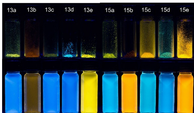
Figure 7. Fluorescence of psoralen derivatives 13 (left) and 15 (right) in solid state (upper row) and dichloromethane (lower row, c(\mathbf{13}), c(\mathbf{15}) = 10^{-7} M, hand-held UV-Lamp, \lambda_{\text{exc}} = 365 nm).
