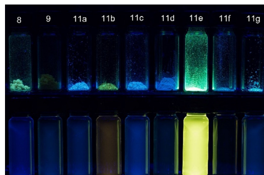
Figure 5. Fluorescence of psoralen derivatives 8 , 9 and 11 in solid state (upper row) and in dichloromethane (lower row, c(\mathbf{8}) , c(\mathbf{9}) , c(\mathbf{11}) = 10^{-7} M , hand-held UV-Lamp, \lambda_{exc} = 365 nm).
