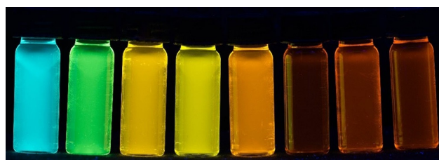
Figure 9. Fluorescence of compound 15e in solvents of different polarity (from left to right: cyclohexane, toluene, chloroform, ethyl acetate, dichloromethane, dimethyl sulfoxide, N,N -dimethylformamide, acetonitrile; \lambda_{\text{exc}} = 365 nm).
