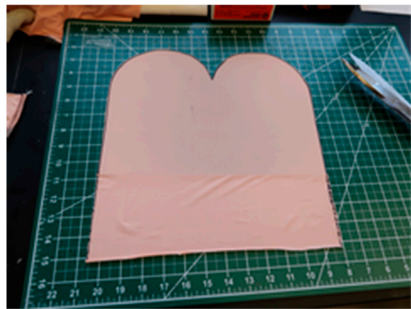
Example of the TOP of the construct after trimming to size. This will be the outer facing side of the Ferrous Liner.
