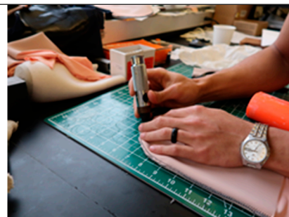
Lay the RLiner construct with now-attached fabric backing flat on the punch mat. Get a 12 mm size punch and use it to punch a hole in the center distal end of the RLiner construct. This is where the pin will protrude from the liner. Using a mat as a measuring tool is useful.
