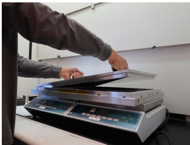
Figure 2. Mold on hotplates. Top lid being positioned in place.
