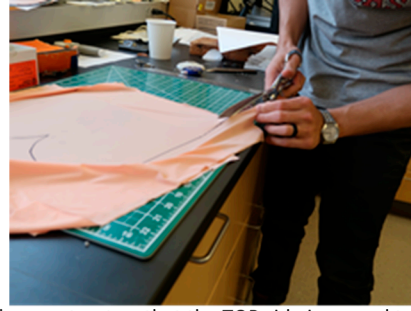
Flip the construct so that the TOP side is up and trim to the Sharpie marks from earlier, starting with the straight edges and meeting in the middle, between the round edges. Use the liner scissors. It is important to leave the Sharpie marks as they are used to sew in the next step. Do trim right up to the Sharpie.
