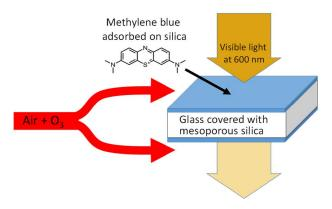
**Figure 1.** Principle of the sensor. A glass slide is covered on both sides with a mesoporous silica thin film on which methylene blue is adsorbed. Visible light at 600 nm is absorbed by this colored material. Exposure to  $O_3$  in the atmosphere leads to an immediate degradation of the dye. The kinetic of absorbance decrease is immediately translated to a concentration.
