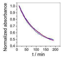
**Figure 4.** Experimental (blue) and model (red) curves of the normalized absorbance as a function of time in the presence of 120 ppb for three sensors analyzed at Day 1, Day 2, and Day 50  $(k_0 = 8.1 \times 10^{-5} \text{ ppb}^{-1} \text{ min}^{-1} \text{ and } A_{inf} = 0.137 \pm 0.003)$ .
