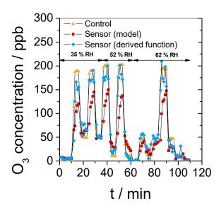
**Figure 7.**  $O_3$  concentration measured as function of time with a benchtop  $O_3$  analyzer for control (triangle) and the sensor using Equation (3) (square) or the derivative as a function of time (Equation (4), lozenge). In this scenario, the  $O_3$  concentration was varied every five to ten minutes from 0 to 10 or 50 or 200 ppb, and the relative humidity in air was changed from 35% to 52% and, finally, 62%.
