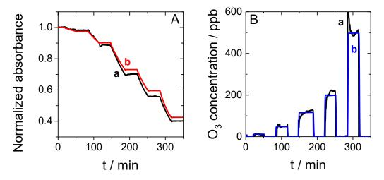
**Figure 5.** (A) Experimental (a, black) and model (b, red) curves showing the normalized absorbance as a function of time in the presence of increasing concentrations of  $O_3$  from 12 to 500 ppb. (B)  $O_3$  concentration measured as a function of time with the  $O_3$  sensor (a, black) and controlled values given by a benchtop  $O_3$  analyzer (b, blue).
