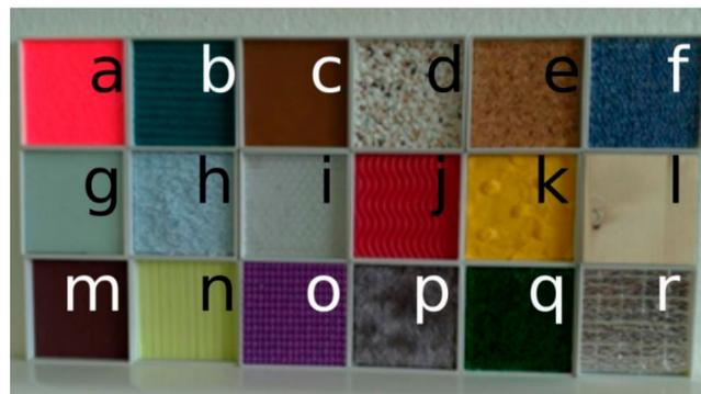
**Figure 21.** Layout of tested specimens: a—felt, b—office carpet (wave pattern), c—leatherette, d—bubble relief styrofoam, e—cork, f—office carpet, g—polyurethane foam, h—carpet with short fibres, i—anti-slippery matt, j—soft foam with wave pattern, k—felt with pattern, l—spruce wood, m—sandpaper, n—wallpaper, o—bubble foam, p—plush, q—fake grass, r—aluminum thermofoil.
