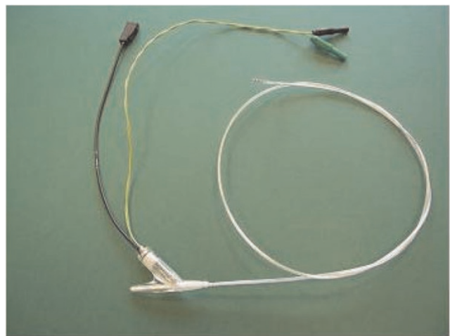
Diagnostic RF-safe MR-EP catheter.
