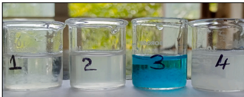
Fig. 4. Beaker 1-Alcohol test, Beaker 2-Citric acid and Sugar solution test, Beaker 3-Fehling solution test and Beaker 4-Lead acetate test.
