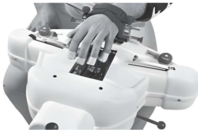
Figure 1 End traction-driven finger rehabilitation machinery.
