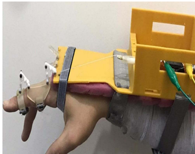
Figure 14 Electroactive material-driven finger rehabilitation machinery.
