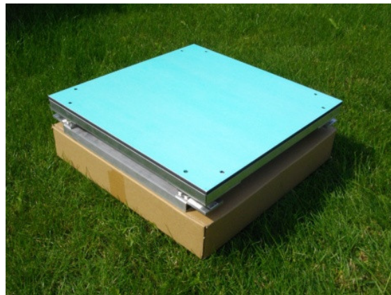
Figure 2. View of the designed electronic beehive scale placed on the ground [16].
