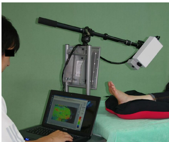
FIGURE 4 Laser speckle flowgraph can measure wounds in a non-invasive and non-contact manner
