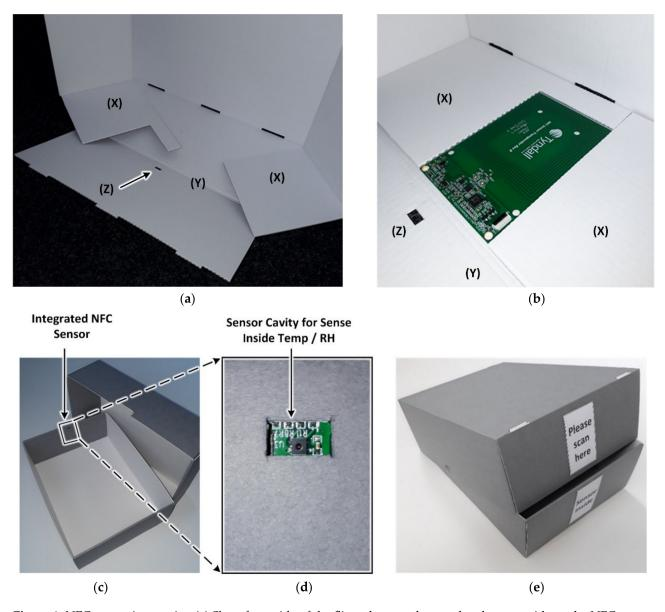
**Figure 6.** NFC sensor integration (a) Short front side of the flipped open telescope box bottom without the NFC sensor, (b) with integrated NFC sensor (c) integrated view of NFC sensor (d) view of sensor cavity for sensing inside temp/RH, and (e) labelled base and lid displaying construction assembly for reading.
