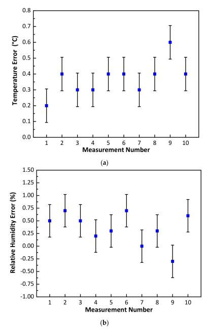
**Figure 8.** NFC sensor measurement comparison with a calibrated Fluke 971 meter (**a**) temperature error (°C) and (**b**) Relative humidity error (%).
