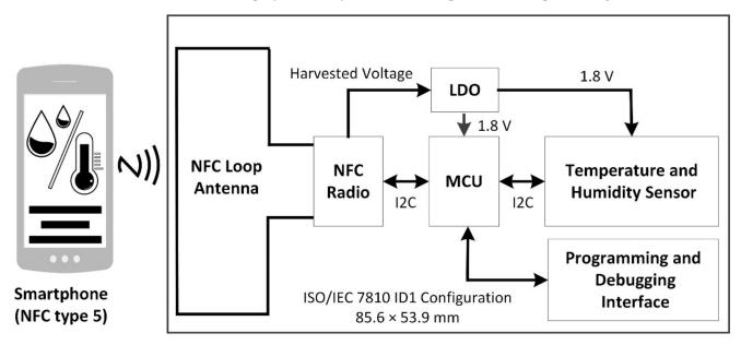
Figure 2. Block diagram of proposed NFC sensor that is powered using a smartphone.
