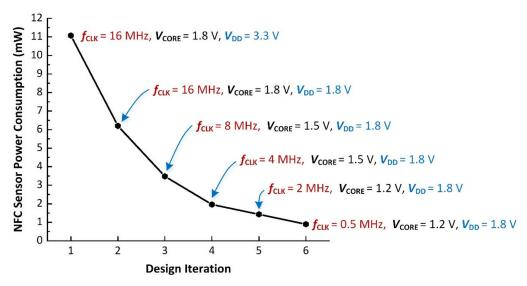
Figure 9. Measured NFC sensor DC power consumption using MCU voltage and frequency scaling.
