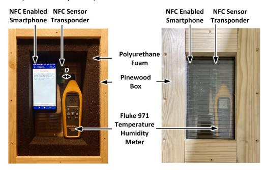
Figure 7. NFC sensor temperature and relative humidity measurement setup.
