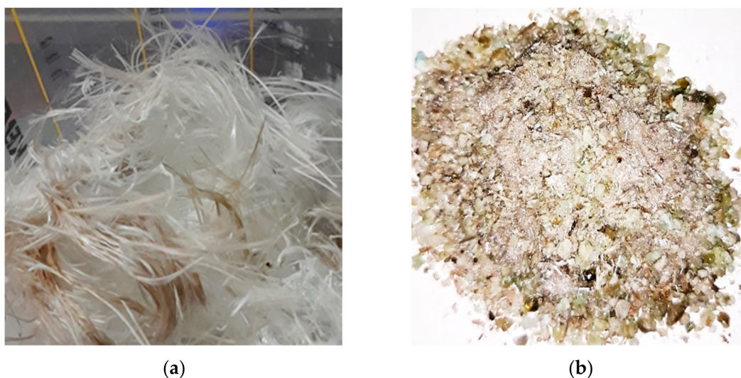
Figure 1. (a) Fiberglass waste; (b) fiberglass waste vitrified with hydrogen plasma.
