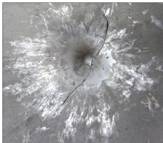
Figure 4: Titanium implant without penetration after shooting with the 9 mm Luger pistol
