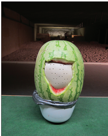
Figure 1: CAD cranioplasty mounted in a water melon on a semi-rigid rack
