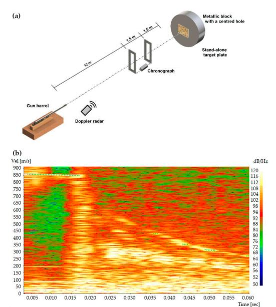
**Figure 2.** (a) Schematic illustration of the CAEx shooting line for stand-alone ballistic test with 7.62 mm ammunition; (b) Actual computer-recorded image (radar spectrum) of projectile velocity variation with time also presented.
