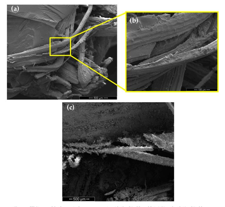
**Figure 9.** SEM image of the damage in the epoxy composite with 15 vol% of fique fabric (**a**,**b**); and with 40 vol% of fique fabric (**c**).
