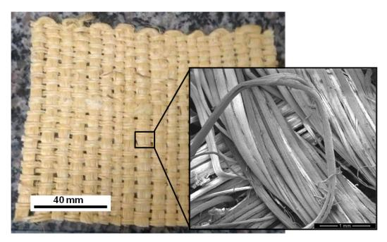
Figure 1. Plain woven fique fabric and microscopic inset of weaved fibers (adapted from [18]).
