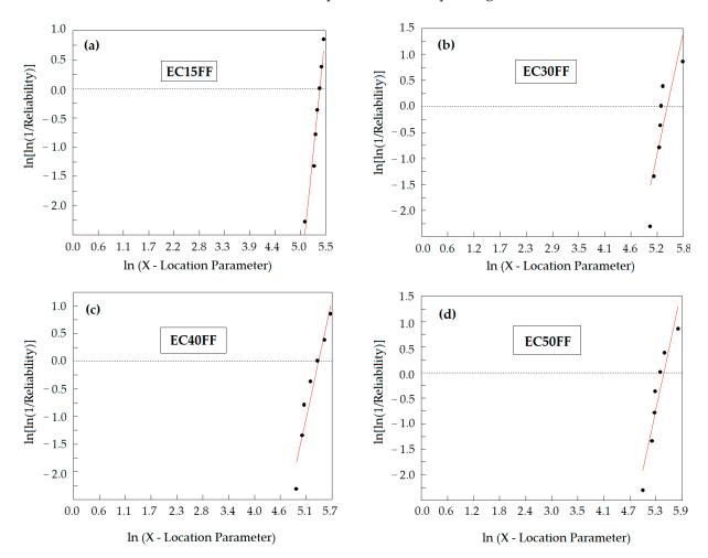
**Figure 5.** Weibull graphs of the stand-alone absorbed ballistic energy ( $E_{abs} \equiv x$ ) for the investigated epoxy composites with: (a) 15 vol%; (b) 30 vol%; (c) 40 vol%; and (d) 50 vol% fique fabric.
