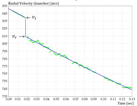
Figure 3. Experimental points obtained from the radar spectrum and the FFT curve fitting.
