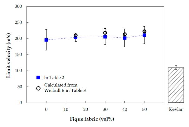
**Figure 7.** Variation of  $V_L$  with the volume fraction of fique fabric from values in Table 2 and calculated from Weibull  $\theta$  in Table 3. Reported  $V_L$  value for Kevlar<sup>TM</sup> indicated in adjacent bar [24].
