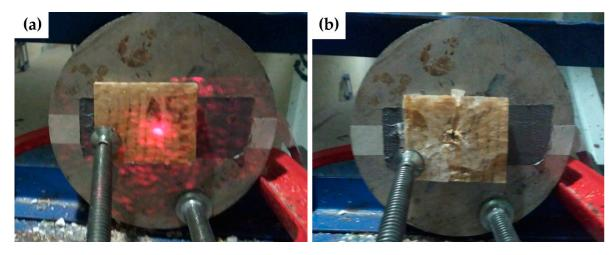
**Figure 4.** Typical stand-alone ballistic test: (a) before shooting, laser beam indicates the direction of 7.62 mm projectile with target plate clamped to a round metallic block; and (b) after shooting, there is perforated hole at the center of the plate.
