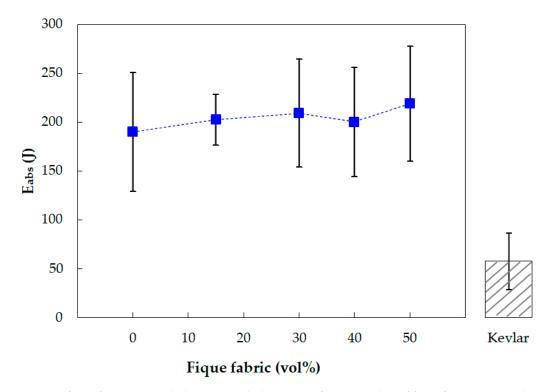
**Figure 6.** Variation of  $E_{abs}$  from the stand-alone test with the volume fraction (vol%) of fique fabric. Reported  $E_{abs}$  value for Kevlar<sup>TM</sup> indicated in adjacent bar [24].
