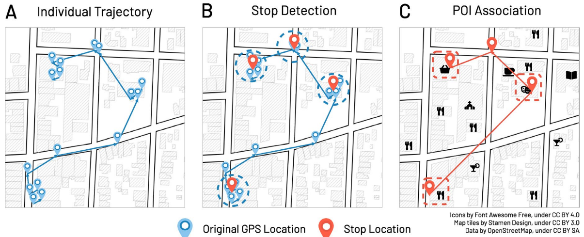
Figure 1. (A) From an individual's original GPS trajectory, we detect a stop whenever the individual spends at least 5 minutes within a distance of 65 meters from a given trajectory point. (B) We detect stop locations through a combination of the Lachesis 37 and DBSCAN algorithms 38 . (C) If present, we associate each stop location to the nearest Point Of Interest (POI) within a distance of 65 m.
