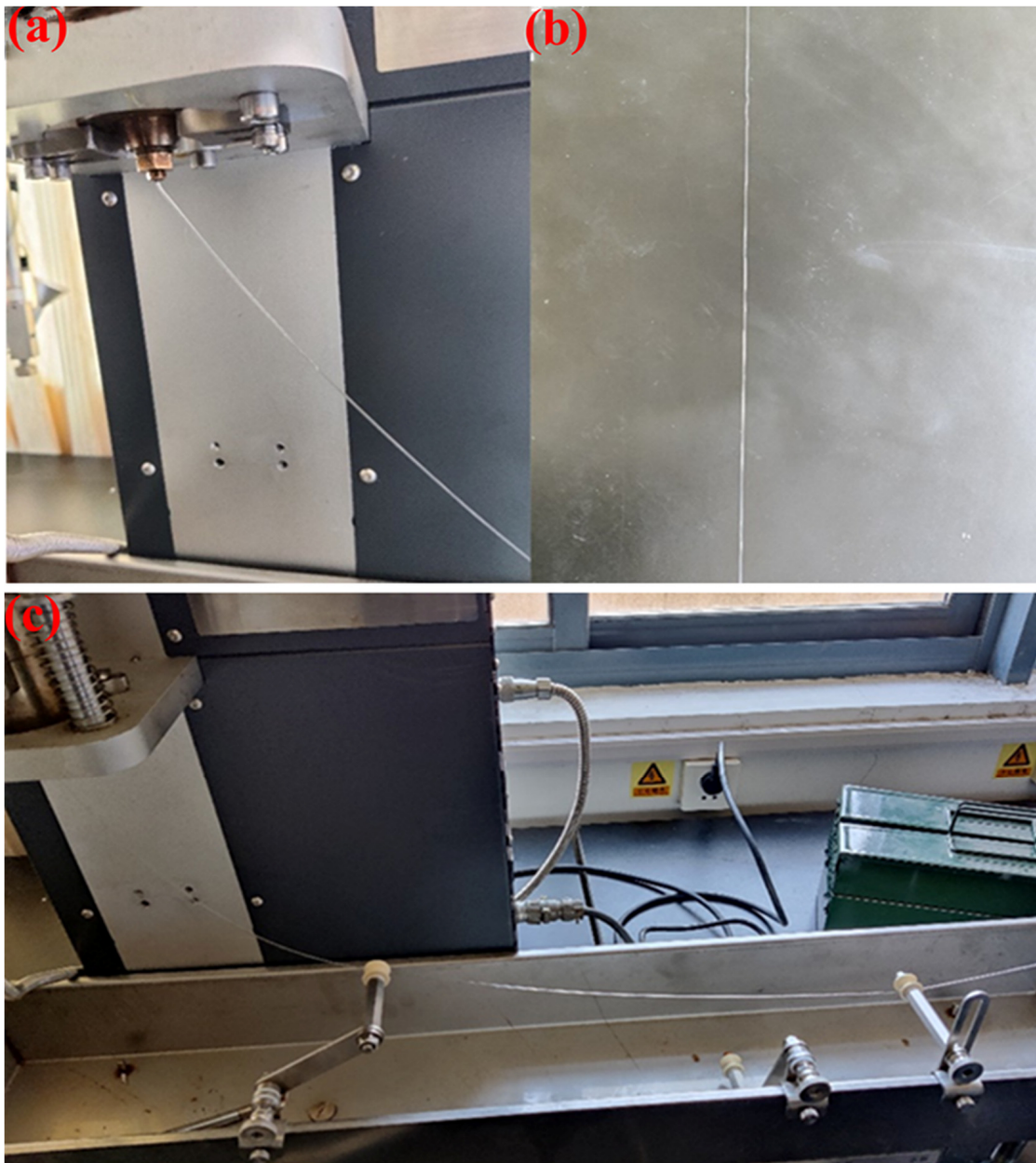
Figure 2. Equipment for melt spinning and drawing: (a) nozzle of melt spinning machine, (b) YAG ceramic fiber cooling in air, (c) drawing mechanism and forming process.
