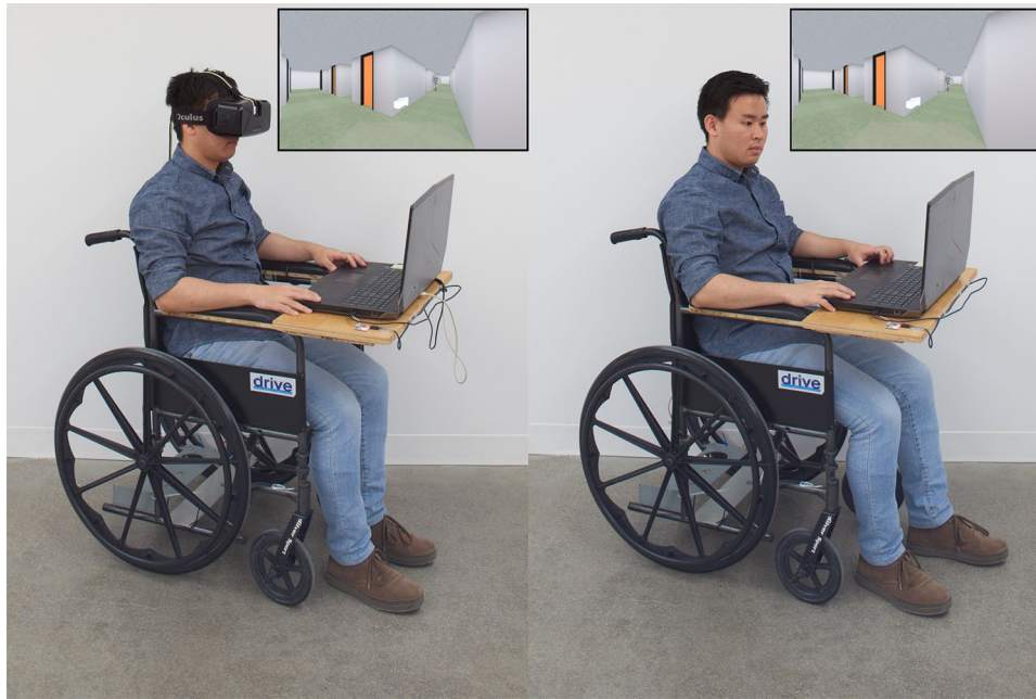
Figure 3. Two experimental setups: using a head-mounted display (left) and a laptop screen (right). The insets depict an example of the virtual environment that the participants observed.
