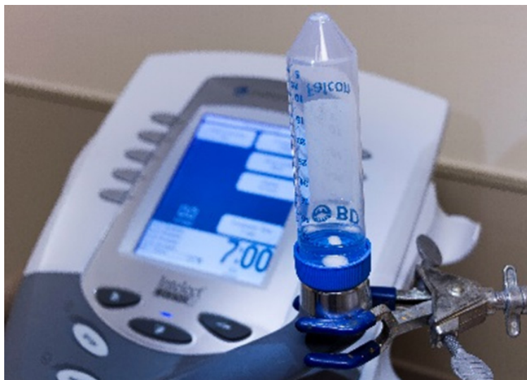
Figure 1. A cement sample is shown undergoing ultrasound (US) treatment. The specimen is kept in its vial and placed directly on the transducer head with a thin layer of US gel.
