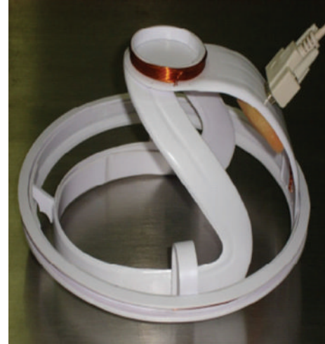
FIGURE 1: Brain injury detector based on Volumetric Electromagnetic Phase Shift Spectroscopy. Courtesy of UC Berkeley.
