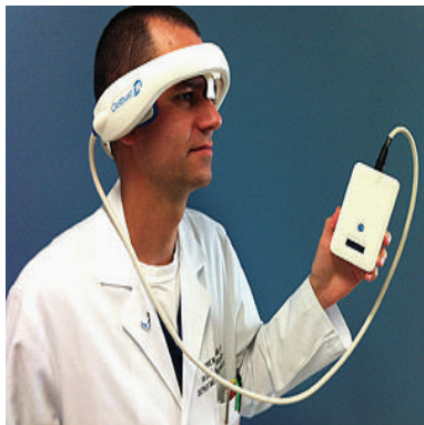
FIGURE 3: The Clotbust ER ultrasound system for thrombolysis. Courtesy of Cereveest Therapeutics Inc.
