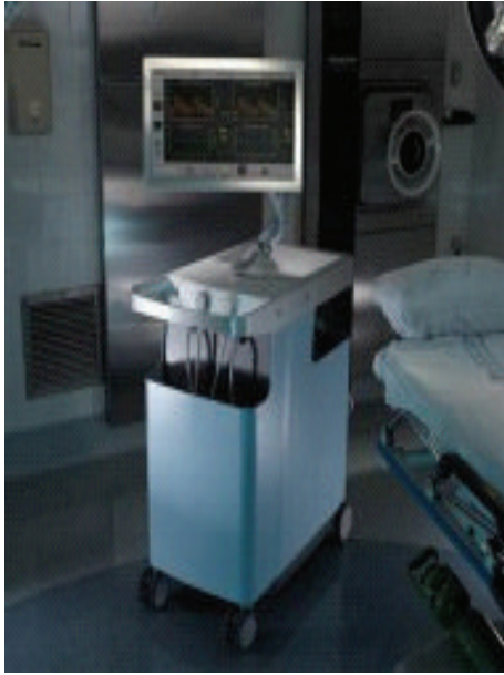
FIGURE 5: The “Presto” Cranial blood flow monitor. Courtesy of Physiosonics.
