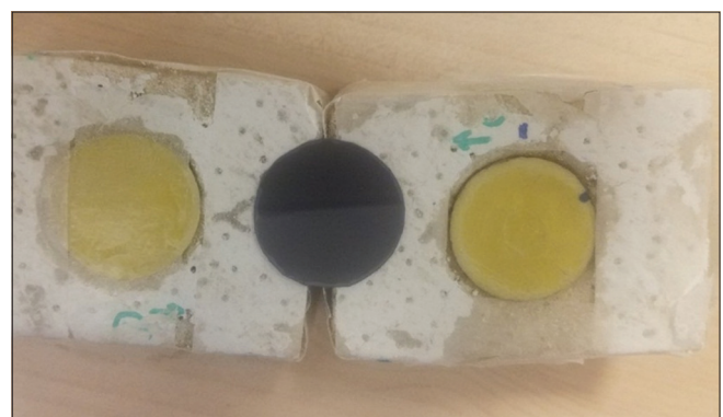
Figure 3: Treatment volume represented by the tumor (two yellow semicircles, left and right), inserted into a cube with mineral fiber and a black circle (in the middle) presenting an irradiated EBT3 dosimetry film
