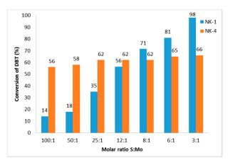
**Figure 4.** Effect of amounts NK-1 and NK-4 on conversion of dibenzothiophene (DBT). Reaction conditions: initial sulfur content 500 ppm, 5 mL of model mixtures, molar ratio  $H_2O_2$ :S = 4:1, 1 mL MeCN, 50 °C, 1 h.
