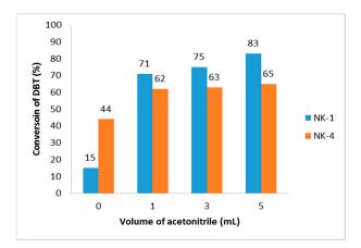
**Figure 6.** Effect of the acetonitrile amount on the conversion of the DBT. Reaction conditions: initial sulfur content 500 ppm, 5 mL of model mixture, molar ratio  $H_2O_2$ :S 4:1, molar ratio S:Mo 8:1, 50 °C, 1 h.
