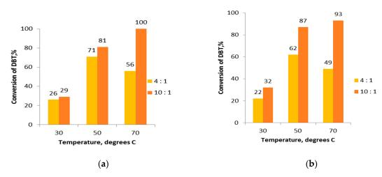
**Figure 7.** Effect of temperature on the conversion of the DBT in the presence of NK-1 catalyst (**a**) and NK-4 catalyst (**b**). Reaction conditions: initial sulfur content 500 ppm, 5 mL of model mixture, molar ratio S:Mo 8:1, molar ratio  $H_2O_2$ :S 4:1, 1 mL MeCN, 1 h.
