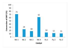
**Figure 3.** Conversion of dibenzothiophene over various catalysts. Reaction conditions: initial sulfur content 500 ppm, 5 mL of model mixture, molar ratio  $H_2O_2$ :S = 4:1, molar ratio sulfur: molybdenum 8:1, 1 mL MeCN, 50 °C, 1 h. Conversion of dibenzothiophene without catalyst is 7%.
