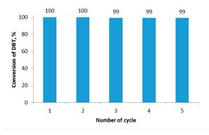
**Figure 9.** Effect of recycling NK-1 on the conversion of DBT. Reaction conditions: initial sulfur content 500 ppm, 5 mL of model mixture, molar ratio H<sub>2</sub>O<sub>2</sub>:S 10:1, molar ratio S:Mo 8:1, 1 mL MeCN, 70 °C, 1 h.
