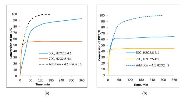
**Figure 8.** Effect of the oxidation duration on the conversion of the DBT in the presence of NK-1 catalyst (**a**) and NK-4 catalyst (**b**). Reaction conditions: initial sulfur content 500 ppm, 5 mL of model mixture, NK-1 as catalyst, molar ratio H<sub>2</sub>O<sub>2</sub>:S 4:1 (10:1), molar ratio S:Mo 8:1, 1 mL MeCN.
