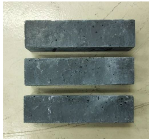
Figure 4. Prism samples for flexural strength tests.
