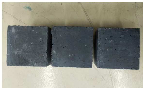
Figure 2. Cubic samples for unconfined compressive strength tests.
