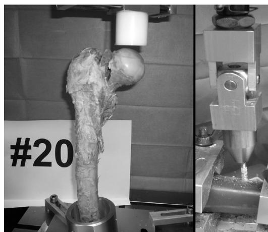
Figure 1. Material testing. A. Pauwels III fracture of a human cadaveric specimen after axial loading. The bone was fixed in a metal cylinder. Axial compression was performed via an artificial acetabulum. B. Osteosynthesis failure after pullout testing of a cortex screw.
