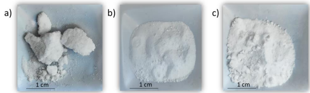
Figure 8. Effect of moisture on physical properties (water absorption) of (a) pure \text{NaNO}_3 , (b) \text{NaNO}_3/\text{SiO}_2 NPs (1% wt.) and (c) \text{NaNO}_3/\text{Al}_2\text{O}_3 NPs (1% wt.).
