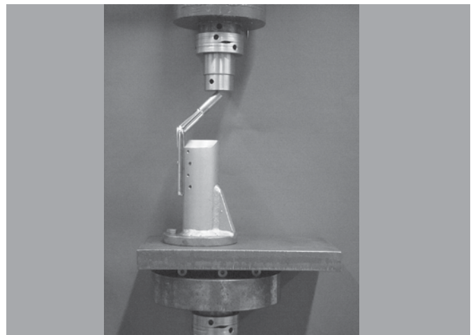
Figure 3. Complete assembly of the device in the angled plate DHS-AF® test®.
