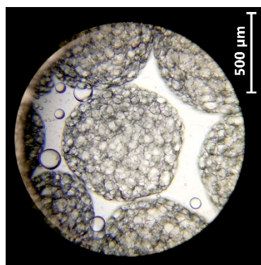
Figure 4. Microscopic image of oil-loaded Ca-alginate beads at a magnification of 10 \times .
