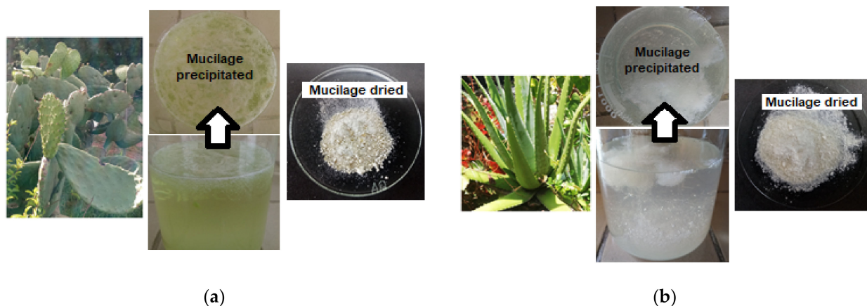
Figure 1. Appearance of the purified mucilage: (a) mucilage extracted from OFI cladodes; (b) mucilage extracted from Aloe Vera leaves.
