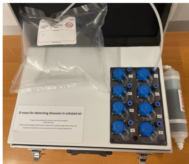
Figure 4. E-nose system used during measurements.
