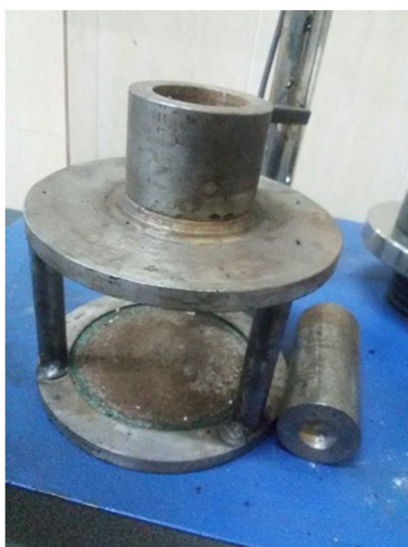
Figure 3. (A) Kim test mold and (B) typical failure modes.3.4. Self-healing Tests.
