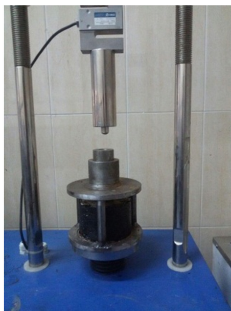
Figure 3. (A) Kim test mold and (B) typical failure modes.3.4. Self-healing Tests.
