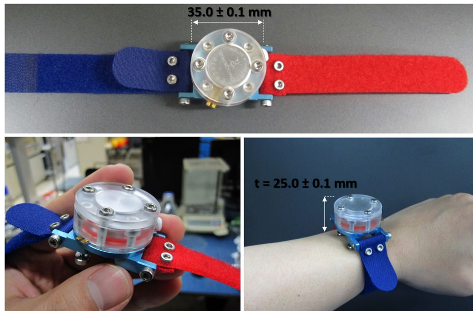
Figure 3. The fabricated watch-type sweat rate sensor.
