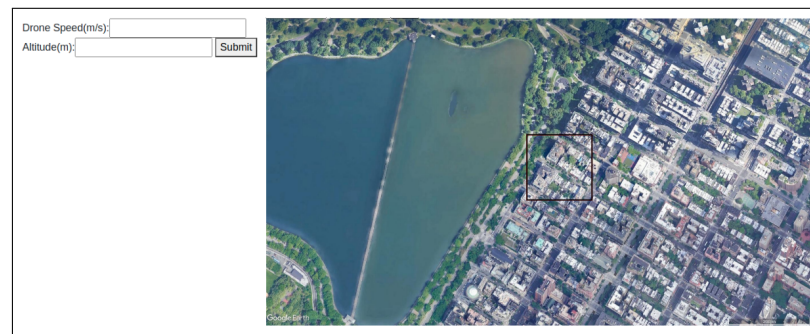
Figure 3. Example of the simulator screen. The drone speed and altitude values are inserted on the left and submitted by the user (by clicking on the “Submit” button); the user clicks on the image and uses the arrows to move the black frame on the map; to finish, the user presses “Enter”.
