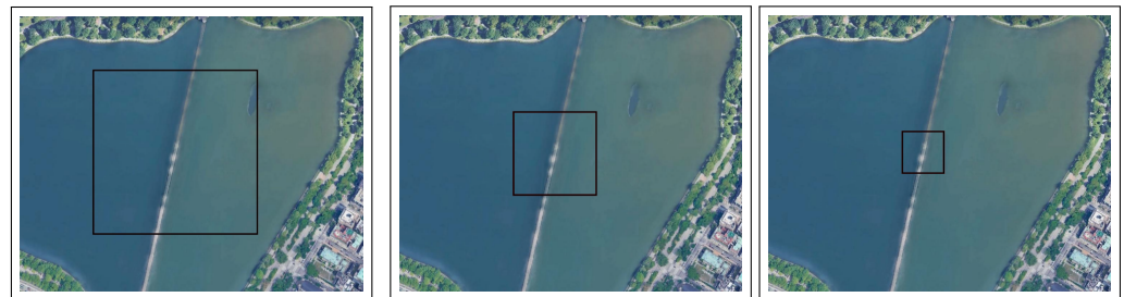
Figure 8. Terrain test for the Central Park Lake location (location #2) from altitudes of: 200 m (in the left image), 100 m (in the center image), 50 m (in the right image).
