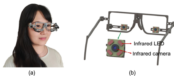
Figure 2. (a) Wearing diagram of the eye tracker. (b) Mechanical structure diagram of eye tracker.
