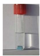
Figure 1. Test tube with gelatin block in complete immersion can be seen
