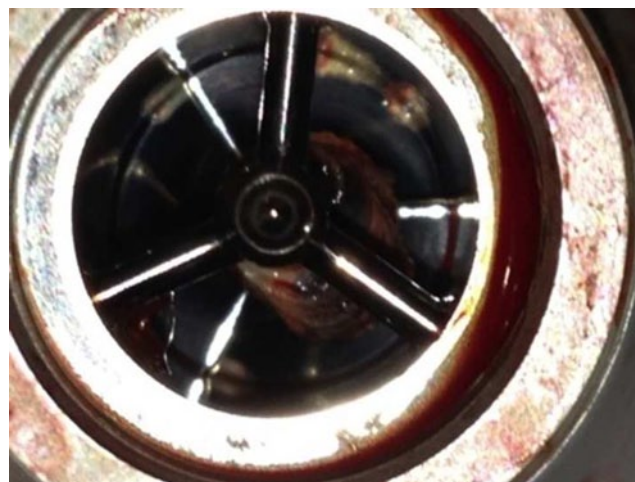
Fig. 2 Thrombus localised on the bearing of the inlet cannula
