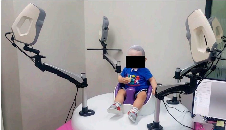
Figure 2. Clinical photograph of the process of scanning for skull deformities. The frequent movement of the infants increased the difficulty of obtaining accurate images. The simultaneous use of four three-dimensional scanners enabled the acquisition of precise images over an imaging duration of only 0.5–0.8 s.
