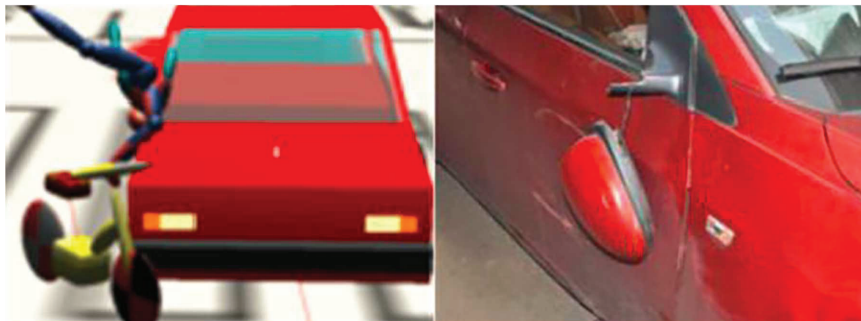
FIGURE 4: Comparison of the relative position in simulation and the damage of the vehicle at 130 ms.
