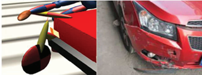
FIGURE 3: Comparison of the relative position in simulation and the damage of the vehicle at 60 ms.
